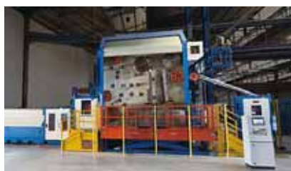
Mario Frigerio large-diameter (13 mm-diameter) copper rod drawing machine and in-line annealer
